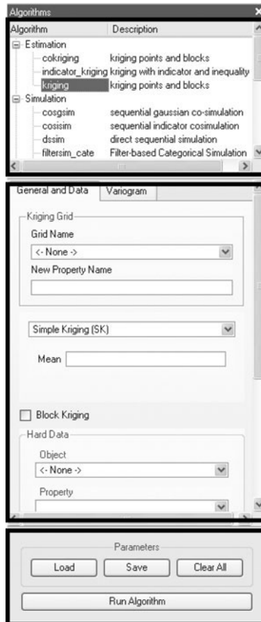
Figure 2.2 The three parts of the Algorithm Panel are highlighted. The top part displays the list of available algorithms. The middle section is where the input parameters for the selected algorithms are entered. The bottom part contains the controls to load/save the algorithms' parameters, and run the selected algorithm
