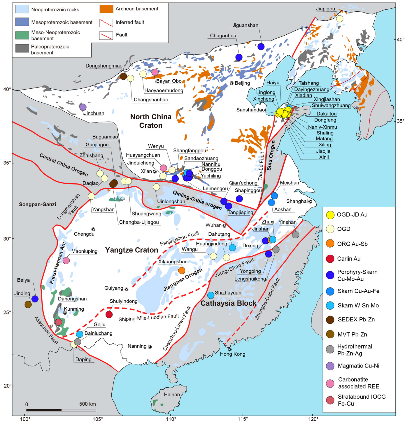
Fig. 19. Tectonic framework of Eastern China showing 66 world-class to giant mineral deposits within ~100 km of the margins of the North China and Yangtze cratons: compiled from multiple sources, mainly within Chang and Goldfarb (2019) . Gold deposits in Qinling-Dabie Orogen classified according to Goldfarb et al. (2019) . From Yang et al. (2021) .
