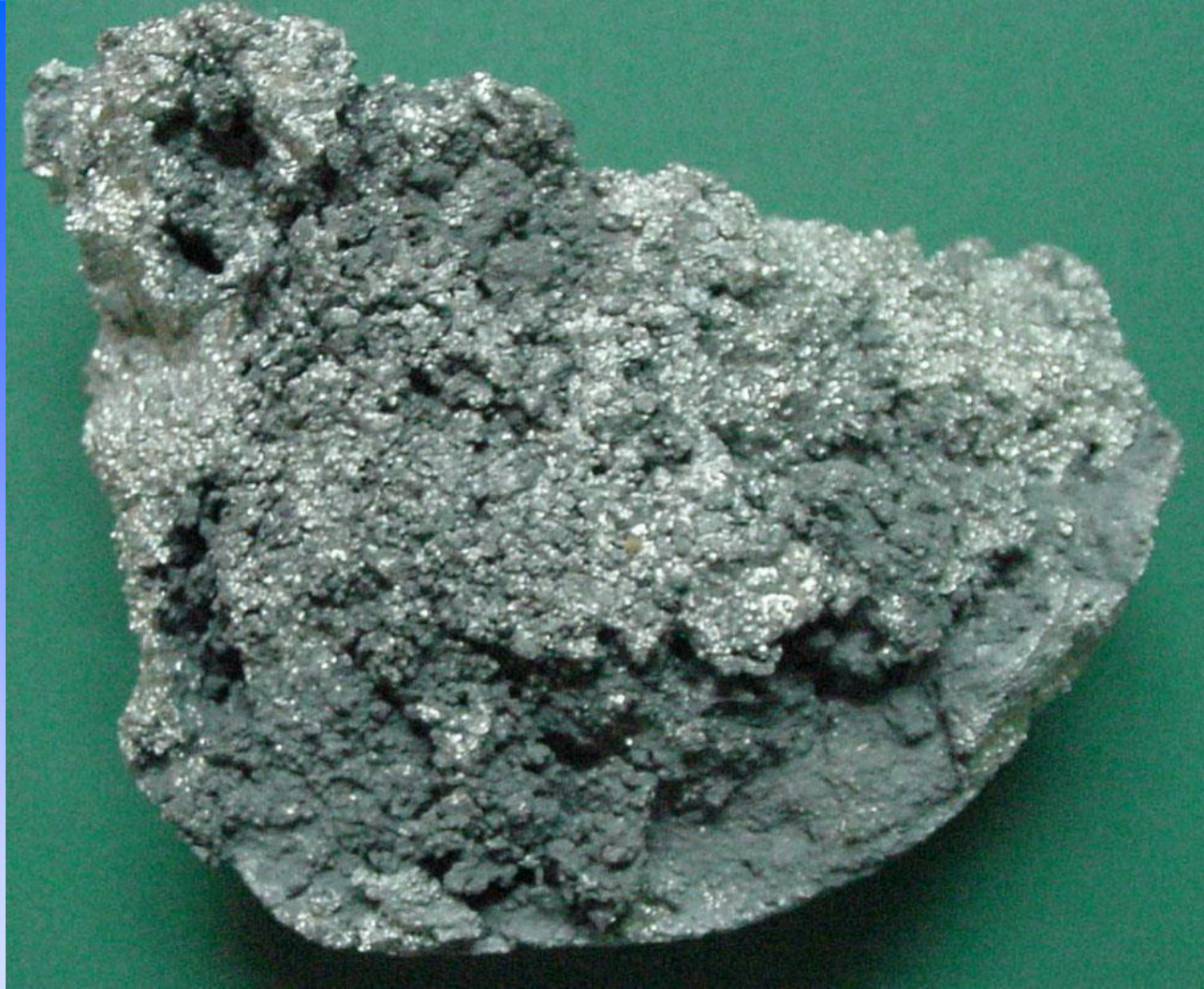
Fig. Bad wetting between as cast Al base matrix and SiC particles.
