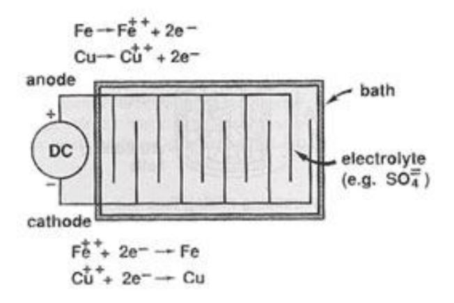
Figure: Electrolytic Cell Operation for Deposition of Powder --- Schematic.
