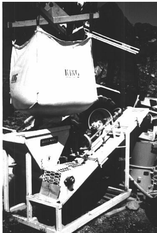
Figure 15.3: Bagged pre-mixed dry shotcrete components being delivered into a hopper feeding a screw conveyor, fitted with a pre-dampener, which discharges into the hopper of a shotcrete machine
