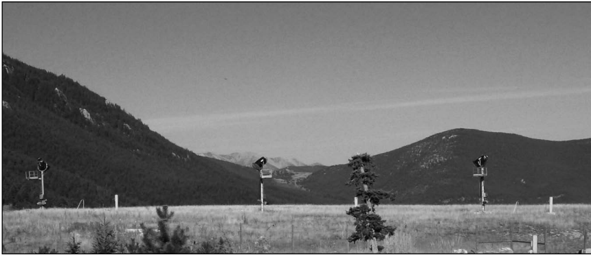
Figure 2. Evaporators/snowmakers can be used to provide a polishing treatment for nitrates and dispose of excess mine waters in the on-site LAD area. The evaporators can be used on uneven terrain to dispose of water by land application in summer and continue to provide disposal and nitrogen polishing treatment by snowmaking in winter (SMC, HKM Engineering Inc., and Knight-Piésold 2004). (DEQ photo)
