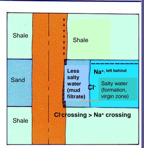
The Na+ ion is comparatively large and drags 4.5 molecules of water, while the CI ion is smaller and drags only 2.5 molecules of water. Hence, the anion CI will migrate more easily than the Na+ ions.
