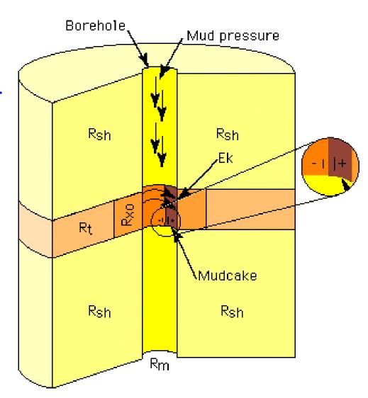
By definition the SSP is the sum of the membrane (E<sub>m</sub>) and junction potential (E<sub>i</sub>)
