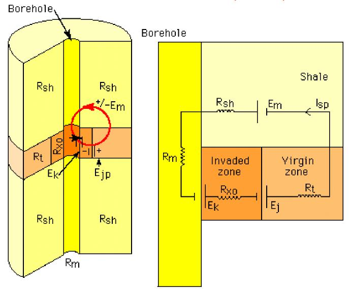
$$E_{D} = \frac{RT}{F} \cdot \frac{v - u}{v + u} \cdot \ln \left( \frac{C_{w}}{C_{mf}} \right) = \frac{RT}{F} \cdot \frac{v - u}{v + u} \cdot \ln \left( \frac{R_{mf}}{R_{w}} \right)$$
